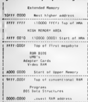
Figure 7-3. Memory Map Showing UMB Region and HMA
